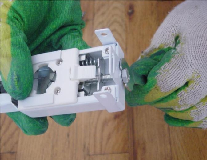
**Check if the Steel Wire is taut enough by pushing it with something. It should not be bent by pushing it and it should be straight and taut. If not, turn the Hexagon Screw more to make sure it is taut.**
