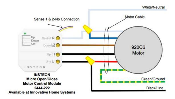
**Note:** If PowerCurtain Remote Control is required to work, PowerCurtain model CL-920C6 Motor will do the job.
